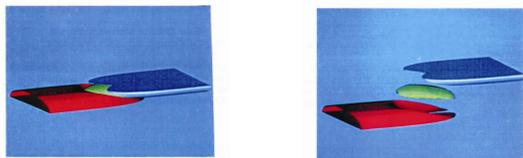
The 3-dimensional groundwater flow field pattern, the flow dynamics and the dimensions of the capture zone, circulation cell, and release zone can be calculated using design aids based on numerical simulations of the groundwater hydraulics.
